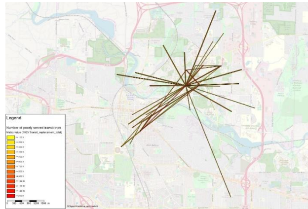
Desire lines showing poorly served transit trips in Ann Arbor
